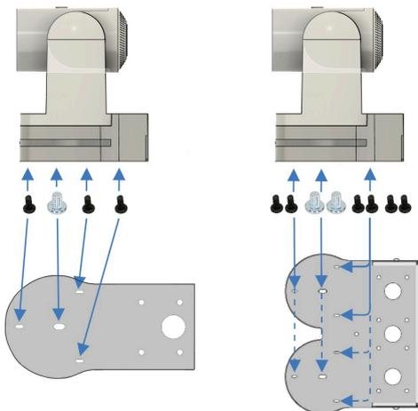
Figure 3: Mounting camera to the baseplate
