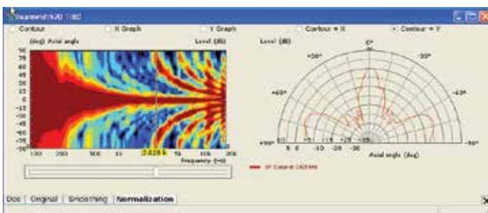
At 3 kHz a very strong side lobes are evident though the main beam is still well defined, this can present many practical problems, not least when working in reverberant spaces.
