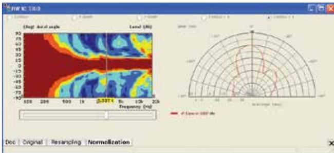
At 3 kHz the beam continues to be well defined with no evidence of aliasing.
