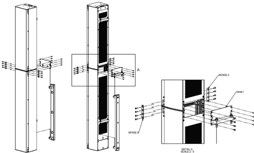
Bracket can be hinged on either side of the cabinet for ease of installation –
