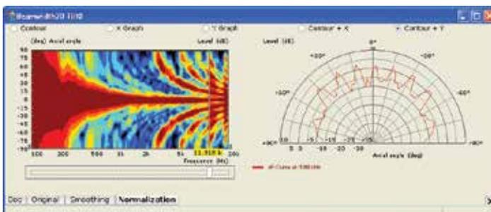
At 12 kHz the directivity characteristics are actually wider than that of a conventional loudspeaker.
