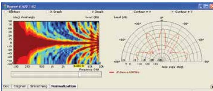
As low as 6 kHz multiple side lobes appear, effective beam control has now collapsed.
