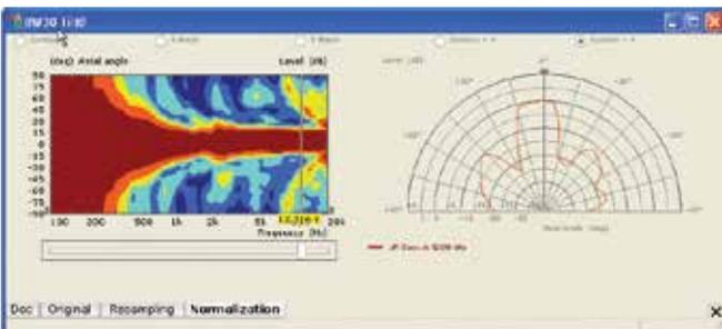
Even at 12 kHz the slight effects of aliasing (which are ultimately and eventually unavoidable) are still 10 dB lower than the main beam.
