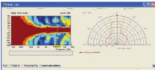
At 6 kHz there is still a well defined beam with no evidence of aliasing being maintained through a much wider range of frequencies than the coax configuration can achieve
