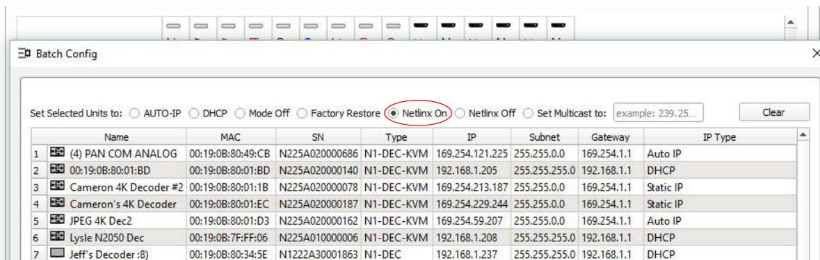
FIG. 25 Enabling NetLinx on Multiple Units
