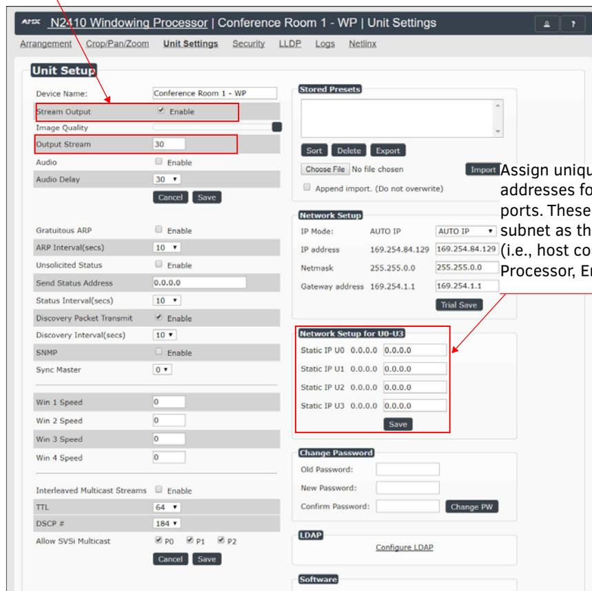
Assign unique static IP addresses for each of the U ports. These must be in the same subnet as the rest of the system (i.e., host computer, Windowing Processor, Encoders, etc.).
