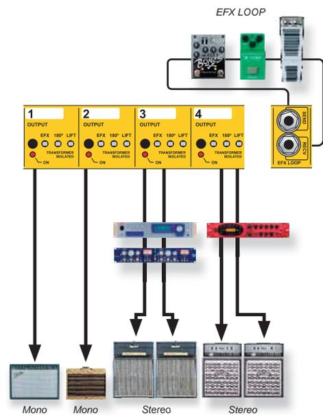
Fig.34 - Setup employs the EFX LOOP as well as dedicated effect processors on the amplifier outputs.
