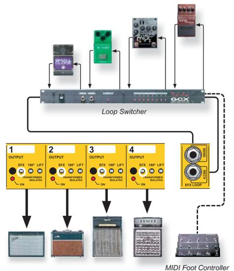
Fig.32 - All amp outputs are assigned to the EFX LOOP. This provides an access point for a multi-loop switcher and MIDI foot controller.
