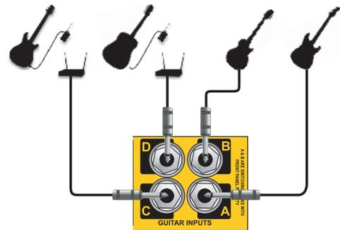
Fig. 15 - Primary input connections on the rear panel.
