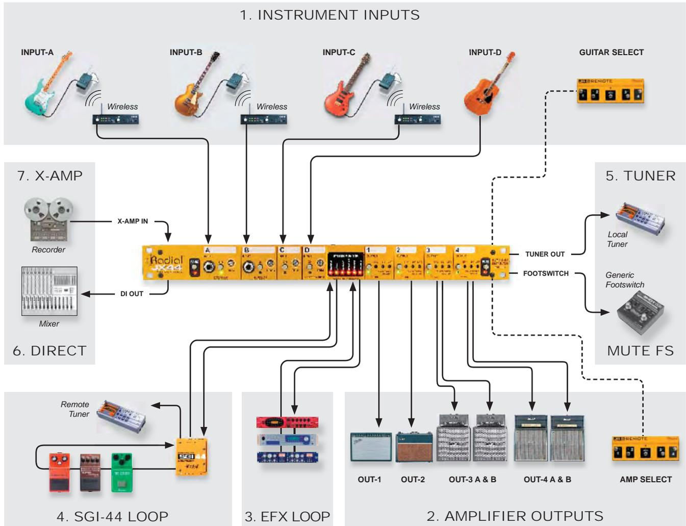
**1. INSTRUMENT INPUTS:** The JX44 starts with a four input instrument selector for wired and wireless guitars. The JX44 can have all your instruments ready and waiting and the optional JR5 remote footswitch allows hands free operation with big, bright LED indicators that are easy to see on stage.
