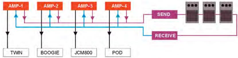
Fig. 11b: The effects loop feeds a bus that the amplifier outputs share.
