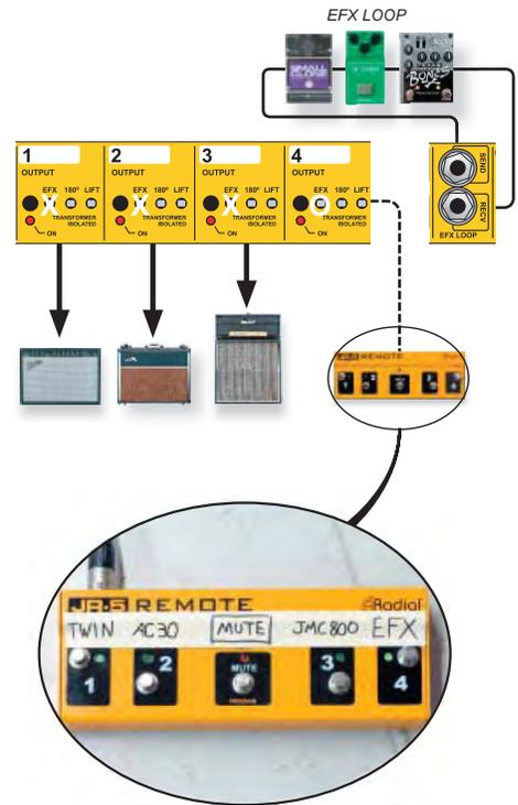
Fig.33 - The JR5 remote footswitch is ideal for this application allowing hands free control of amps and effects.
