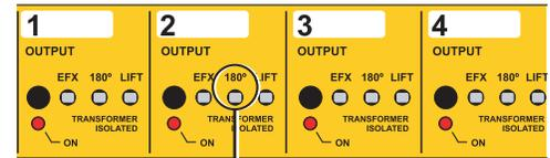
Fig.24 - Outputs 1, 2, 3A and 4A have their 180° controls on the front panel.
