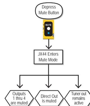
Fig.6 - MUTE mode, all outputs are silenced except the tuner output.
