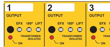
Fig.5b- Separate EFX, 180° and ground LIFT controls on each output allow you to optimize the performance of your amps and system setup.
