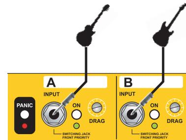
Fig. 2 - INPUTS-A and B on the front panel have priority. When you connect a guitar they will override the rear inputs.
