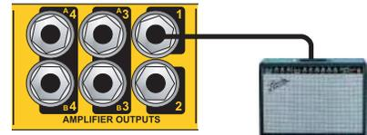
Fig. 18 - Connect an amplifier to OUTPUT-1 to test the instrument inputs.
