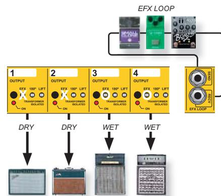
Fig.31 - The first two amps are used without effects for dry rhythm sounds. The other two amps are used with the EFX LOOP for wet leads and special effects.
