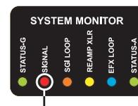
Fig. 20 - This LED indicates when an instrument signal is present at the active input.
