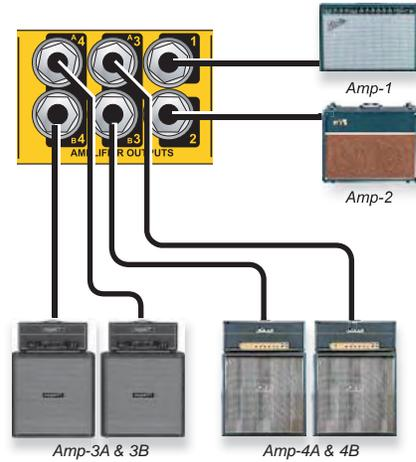
Fig.22 - Up to six amplifiers can be connected using the dual parallel jacks on OUTPUT-3 & 4.
