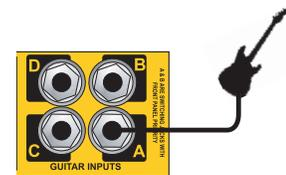
Fig. 19 - Connect an instrument to INPUT-A.
