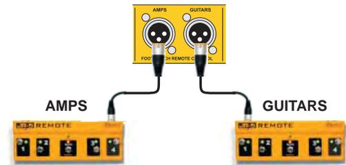
Fig.8 - Two Radial JR5 footswitches may be used at once: one to control guitars and another to control the amps.
