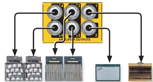
Fig.9 - There are four amplifier outputs on the JX44. Amplifier outputs 1 & 2 are single jacks while outputs 3 & 4 are dual.
