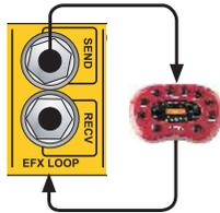
Fig. 11a - The EFX LOOP uses the SEND and RECV jacks on the rear panel.
