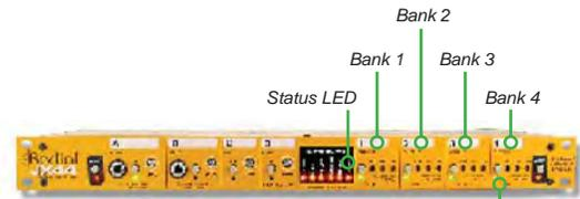
Fig.26 - JX44 BANKS: Hold down front panel MUTE switch for 3 seconds to enter JX44 bank mode.
