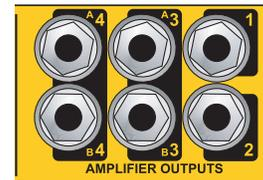
Fig.5a- To keep the front panel clear from obstructions, all amplifier connections are done on the rear. Amplifier outputs 1 and 2 are single while outputs 3 and 4 are dual.
