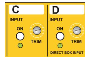
Fig. 3 - Inputs C and D feature TRIM controls to balance the levels of louder instrument signals such as buffered wireless systems and active acoustic guitars with passive instruments.
