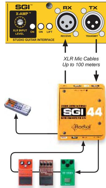
Fig. 14 - SGI LOOP flows out to the SGI-44, through pedal effects, and back to the JX44.
