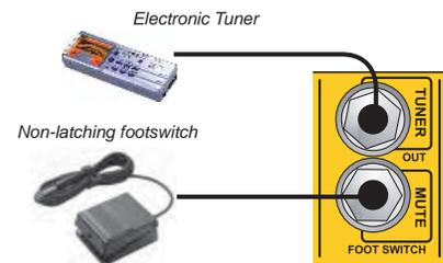
Fig.10 - A separate tuner output keeps clocking noise out of the signal path. The MUTE jack uses a non-latching momentary footswitch.
