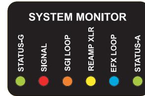
Fig.4 - The JX44 System Monitor provides the status of six functions with easy to see LED indicators.
