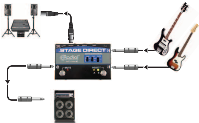
Connections for instrument, stage amp and PA system.
