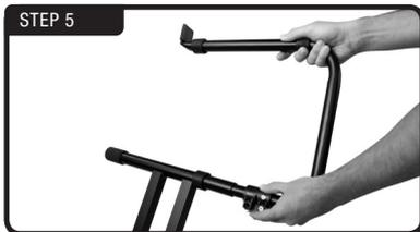
While holding the plastic red triangle, slide the 2nd tier into the top tube.
