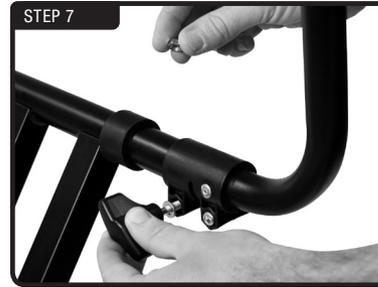
Install hand z-knob, washer, and hex nut. It is important to place the hand knob on the inside or stand will not fold fully. Also, be careful not to over-tighten the hand knobs because over-tightening may cause cracking of the collar.
