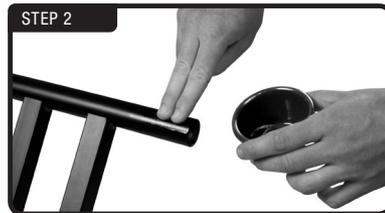
In preparation for STEP 3, use water and soap to lubricate tube.
