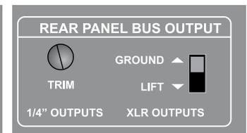
Trim control for the mix bus 1/4" outs and ground lift for the XLR outputs.
