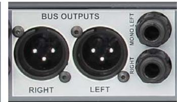
Mix bus includes balanced XLR and unbalanced 1/4" outputs.
