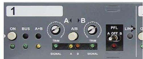
A+B Mix Switch On Channel-1
