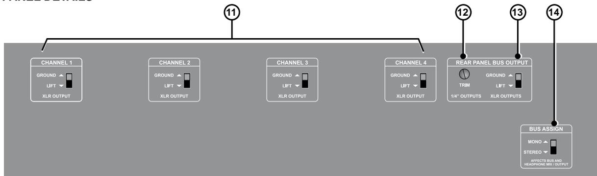
11. **GROUND LIFT:** Disconnects the ground from the channel XLR outputs to eliminate hum and buzz caused by ground loops.
