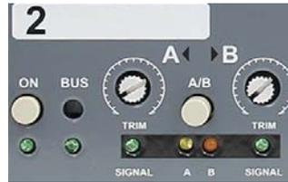
Recessed BUS switch routes the channel output to the mix bus.
