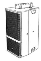
The flybar fits to the top of the MC12-P speaker using two of the existing M10 screws as shown. Securely tighten both screws.
