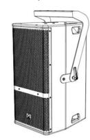
The yoke bracket fits to the sides of the MC12-P speaker, using the existing M10 mounting screws, two per side. Note that the yoke bracket is oriented
