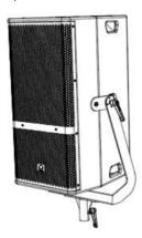
The SA35 bracket attaches to the MC12-P-YB yoke bracket with two screws.
