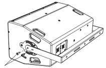
Secure the other end of the swivel bracket with the existing M10 mounting screw as shown. There is a
