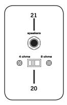
20. IMPEDANCE SELECTOR: Use this switch to match the output impedance of the amp to the speaker(s) being used (4 or 8 ohms).
