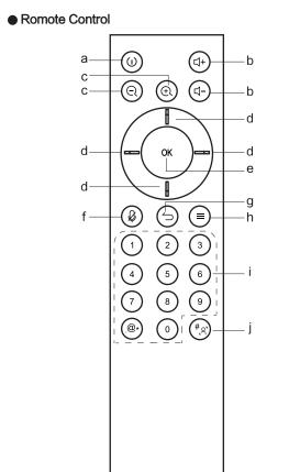
d. Direction Button: Press the direction buttons to move the camera or selection.
