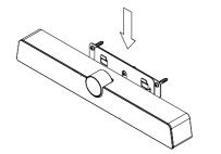
3) Use with panel: Fix the bracket onto the supporting bracket with screws, then place the integrated video conference terminal onto the bracket.(The bracket needs to be purchased separately.)
