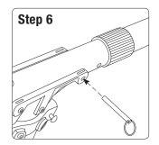
Secure both arms in a horizontal position with locking pins.
