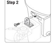
Flip and turn the angle adapter. Screw angle adapter back into the vertical struts.
