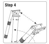
Pull vertical struts upward to a vertical position and spread them to their open position.
