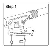
Pull, or rotate, locking pin collar out to release inner strut.
