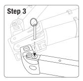
Secure both legs in an open position with locking pins.
