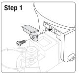
Loosen and remove the screw and angle adapter from vertical struts.
