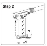
Raise or lower inner strut to desired height and push, or rotate, locking pin collar into locking position.
