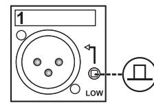
*When using the mPress with an Exo-Pod, the GALLERY OUTPUT should be set to HIGH by disengaging the recessed switch to the OUT position.*
