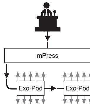
The mPress features two microphone preamplifiers with available 48V phantom power. XLR inputs are paralleled on the front and rear of the unit for convenience. A limiter with adjustable threshold and release controls can be engaged after the mic inputs to reduce the possibility of overloading recorder inputs. The rear XLR inputs can also be set to line level to distribute the outputs of a mixing console or other line level source.
