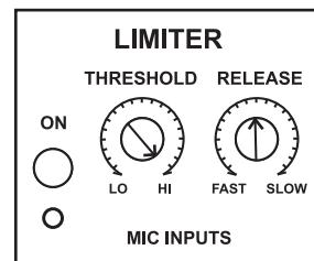
*Start with the THRESHOLD fully clockwise and roll back until loud peaks no longer distort the mic pre.*
