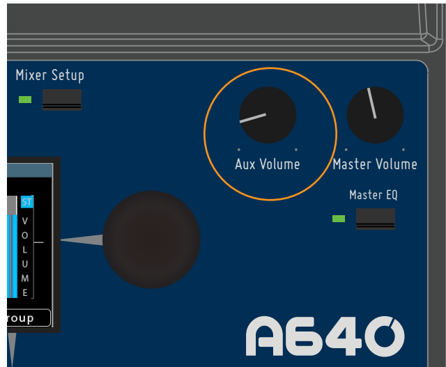
Set the output level of the mono mix with the Aux Volume knob.
