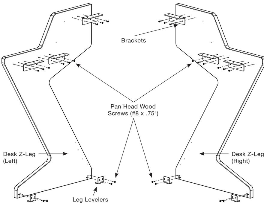
Lay both Z-legs down with holes facing up. Attach three brackets to each of the z-legs. Use three pan head wood screws (#8 x 75") for each bracket. At the base of each z-leg attach leg levelers. Use two pan head screws (#8 x 75") for each of the leg levelers.
