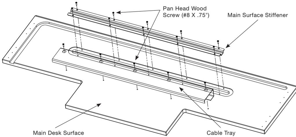
Lay main desk work surface down with groove and holes facing up. In groove place main surface stiffener, the u-shape Stiffener will fit inside the desk groove. Use ten pan head wood screws (#8 X .75") to attach.
