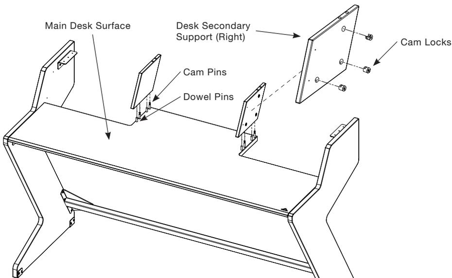
Slide the desk secondary supports onto the dowel rods and cam pins. Place screw driver into cam lock and turn clock wise to lock cam pins in place. (2 each, 4 total)
