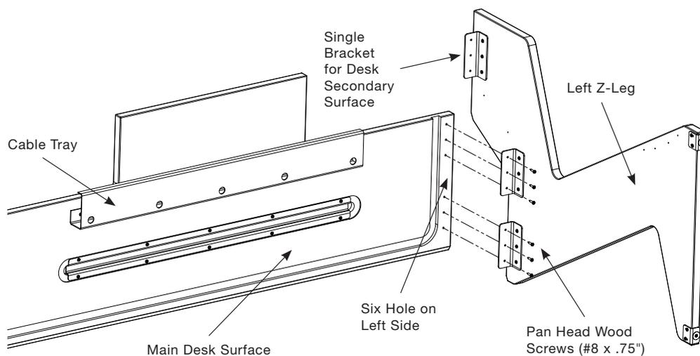
Stand up main desk surface with cable tray at the top. Stand up left z-leg, making sure the single bracket for the desk secondary surface is at the top. Line up the two brackets on the left z-leg with the six holes on the left side of the main desk surface. Use pan head wood screws (#8 X .75") to attach left z-leg to main desk surface. Repeat this with the right z-leg
