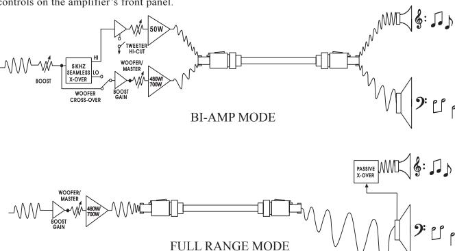
Horn Bi-Amp Mode: This mode requires a GK Horn Bi-Amp compatible bass cabinet. Use a properly wired four-conductor Speakon cable to connect to your cabinet. Set the switch on the back of your GK HBS compatible enclosure to Bi-Amp. In this mode, the cabinet's internal crossover is bypassed. Use the Woofer/Main knob to control the output signal to the woofer, and the Horn knob to control the output signal to the horn.
